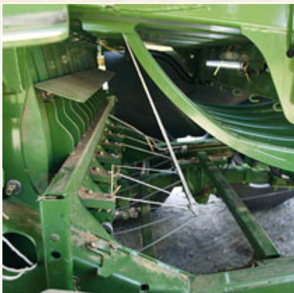
The needles are fairly easy to reach thanks to fold-up twine boxes. LED strip lighting is a big help in the event of a problem at night.
