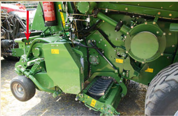
The knife drawer lowers via buttons (arrow). One half then pulls out to the nearside, the other to the offside. The big housing (right) covers the driveline protection clutch for the VFS packer.
