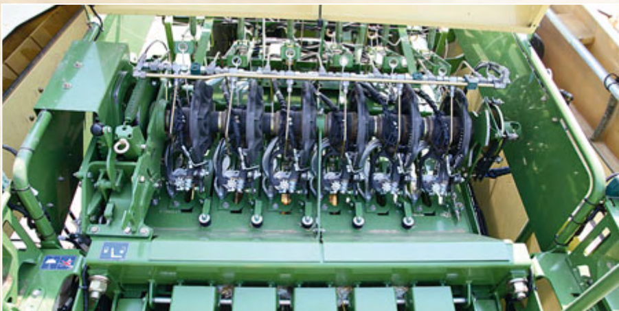
The six double knotters worked reliably but could do with more cleaning airflow in some circumstances. A MultiBale option lets the machine produce up to nine small bales tied into a full-sized pack.
