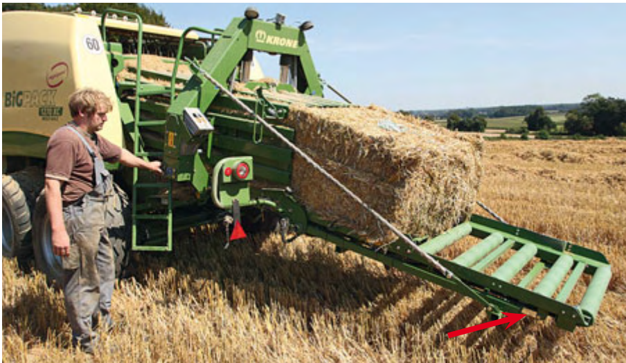
The bale ejector and fold-up chute are button-operated from alongside. Four load cells (arrow) assess bale weight, returning an impressive \pm 2\% accuracy on test.
