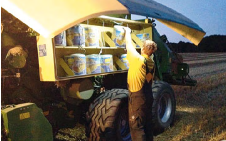
Twine boxes holding 16 balls each are on either side. Optional extra boxes boost total capacity to 44.
