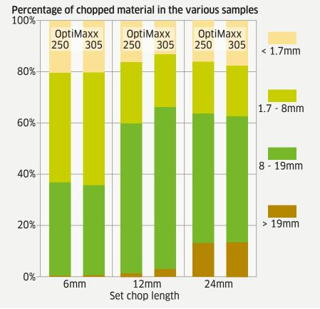
The graph shows that the structure of the chopped material is not really affected by the cracker size. The percentage of coarse material increases when the length of chop is 24mm.
