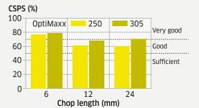
Across all chop lengths, the 305mm cracker delivered higher CSPS scores than the smaller diameter cracker.
