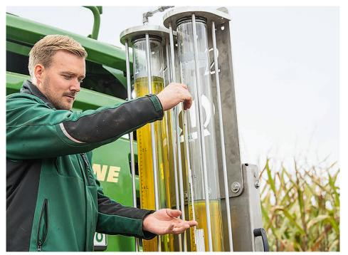
Consumption for each test run was measured with these fuel metering columns.
