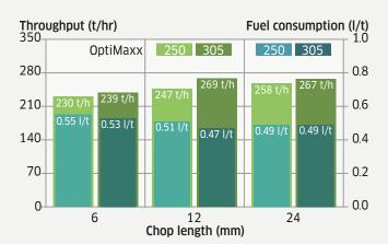
Throughputs averaged to 32% DM. The fuel consumption drops only minimally per tonne when chop length increases. Graphs: Tovornik
